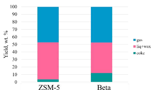
Figure 1. Product distribution over polyisoprene cracking with ZSM-5 and Beta zeolites
